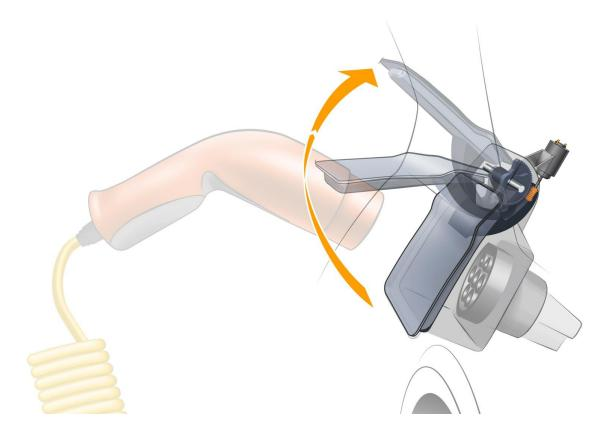
Charging system with a vertically electrical mechanism Concepts for the future
