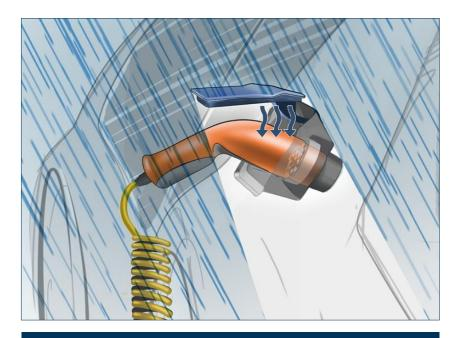
(Infrared) radiant heater for continuous drying during heavy rain, snowfall or ice.
